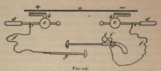
Interrupted Primary Circuit of a Holtz Machine, without Condensers.
